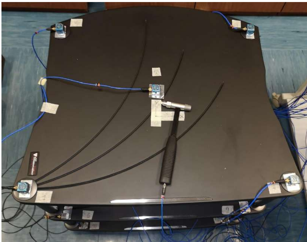
Figure 4. Classic line rack during modal tests – Sensor installation on the top shelf.
